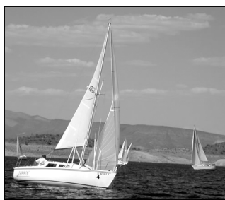
Mast rake is essential in medium to heavy air. Leeches free more easily.
