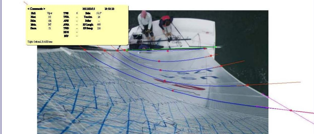
You can see how the EASED OUTHAUL results in a deeper sail at the foot, 25% and 50% heights. Here is nice 3D overlay comparing the **EASED OUTHAUL** and **TIGHT OUTHAUL** setting.
